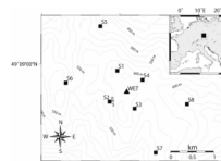
fig.4: Seismic array to determine rotations from translations
