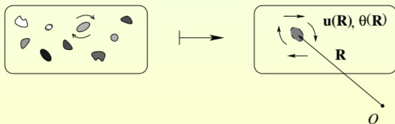
Modelling of a **compressed soil**: An “averaged” particle may rotate and move, the surrounding medium resists to its rotation and motion.
