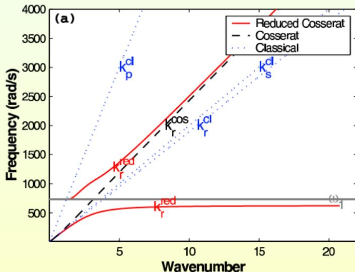
Figure: Numerical example illustrating the behavior of (a) wavenumber, (b) phase, and (c) group velocities for a Rayleigh wave in the reduced Cosserat continuum
