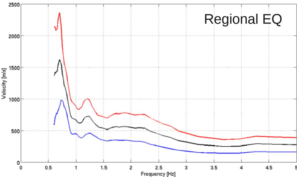
Rayleigh-waves dispersion curve for the MW = 4.9, July 17th, 2011, earthquake. Velocities are obtained through a **linear regression between vertical acceleration and rotation rate**. ZLCC > 0.75.
