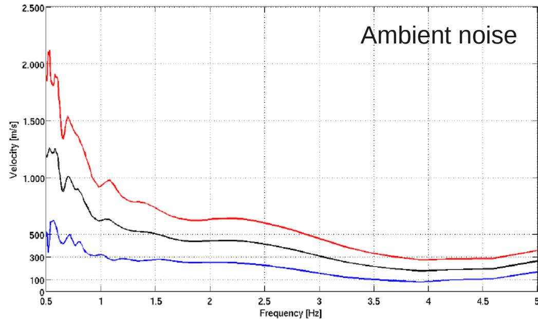
Rayleigh-waves dispersion curve from collocated measurements of rotation and translation for a 5 hours long ambient seismic noise signal. **Linear regression** (ZLCC > 0.75).
